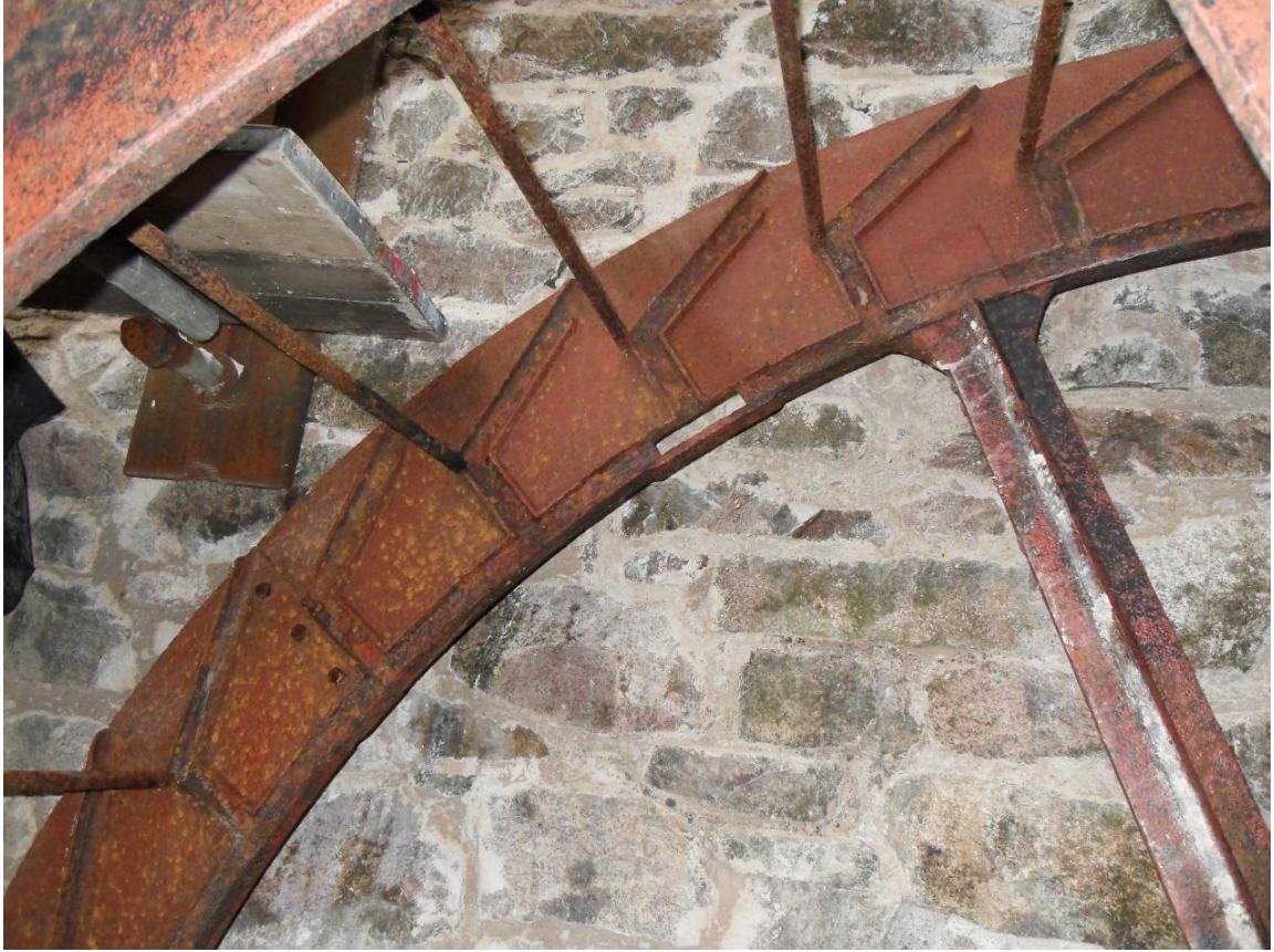
19 Lower waterwheel after rotten timber removal and metal work clean.
