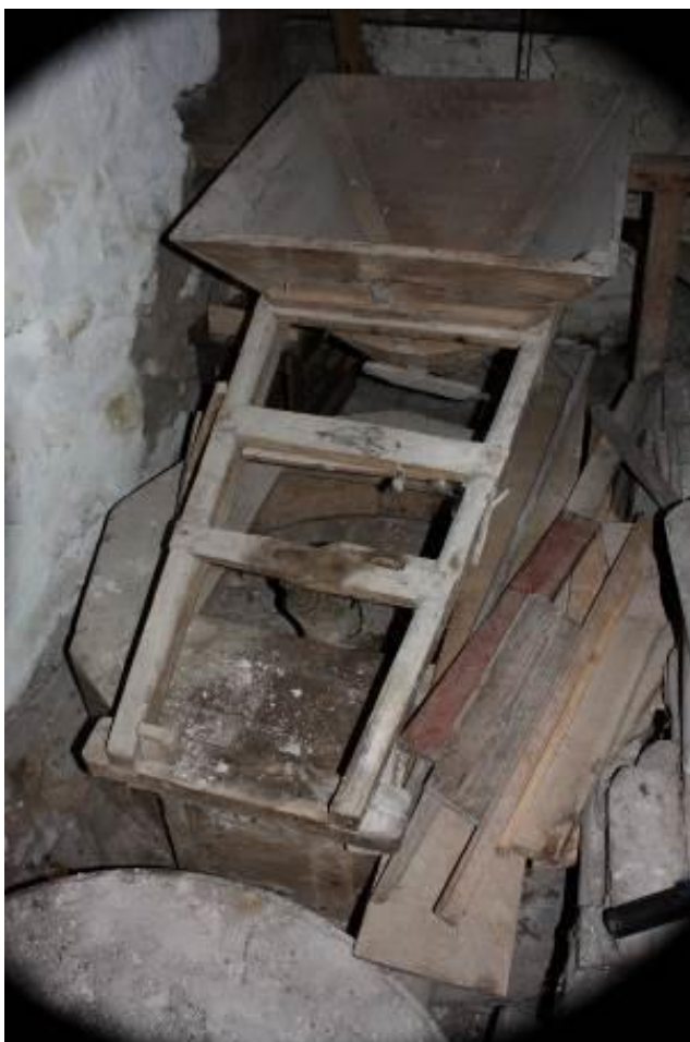
20 An example of the lower millstone furniture before millwright work
